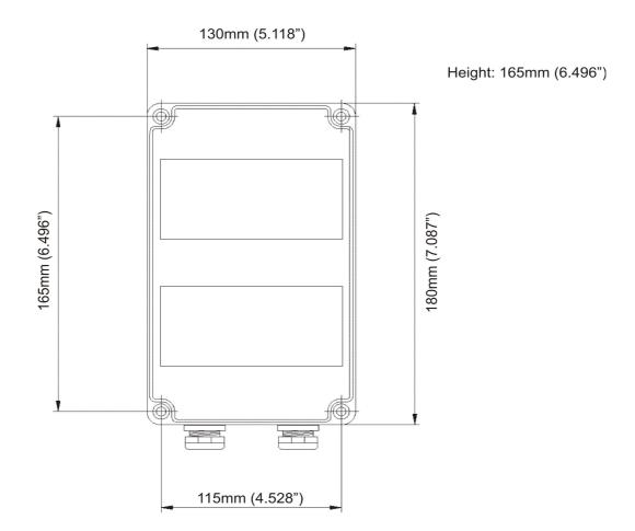
The second panel meter can be installed by simply clipping the blanking plate away with a side cutter.
