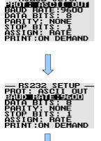
Select the communication protocol. The communication protocol can be set to: "ASCII OUT": A simple ASCII protocol to interface to serial printers and large displays. Please see the format of the ASCII out protocol in section 5.5.1 "MODBUS RTU": Modbus RTU protocol "MODBUS ASC": Modbus ASCII protocol.
