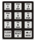
The IQ320 contains a full alpha-numeric keypad for data entry in programing mode. During the normal display mode certain keys have alternate functions. These are:
