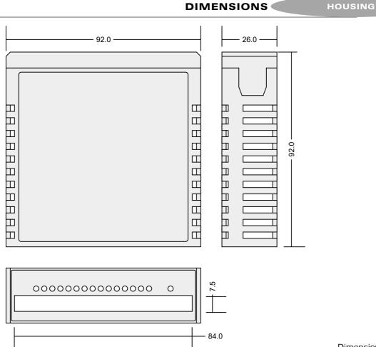
Dimension in mm IP40 rating Rail mount industrial strength single piece housing Rail clips not shown Flame retardant ABS plastic (UL 94 V-0)
